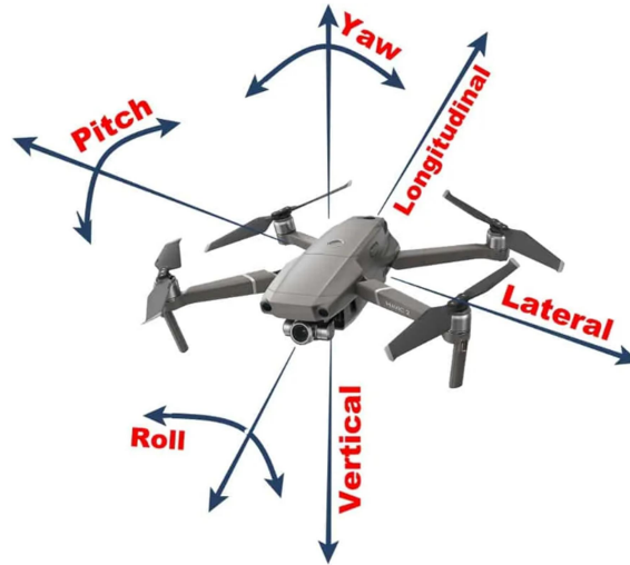
Figure 7 – Flight moves types of drones or quadcopters
