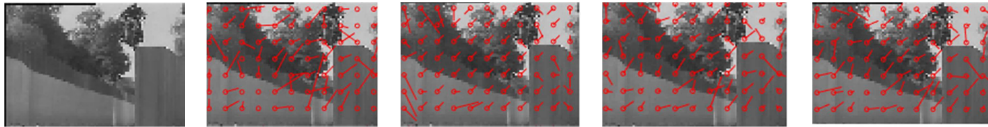
Figure 5 – Proposed Voting Method. From left to right: a. original image, b. optical flow, c. block matching, d. voting approach 1 e. voting approach 2
